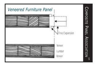
Even minor imbalances in the characteristics of the restraining members can cause significant warping. The greater the potential expansion of the lumber panel, the greater the warp when a restraint is removed on one side.
