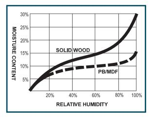
"Expansion or contraction in wood products is directly related to moisture content changes. The degree of movement depends on the expansion/shrinkage coefficient of the product."
