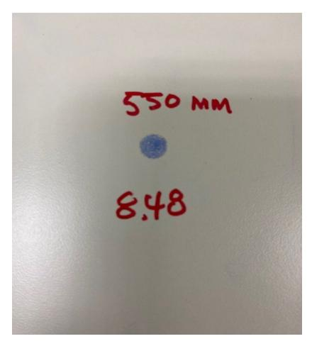
**Figure 3.** Figure 3 illustrates the impact area prior after wiping with isopropyl or acetone making the circle crack more visible.
