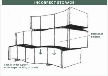
of 3 bottom support bolsters. Bolsters for a given unit must all be of equal thickness. Arrange stacks so that bolsters and top protective strips are aligned and overall stacks are as square as possible. The weight of several thousand pounds of material on panels with misaligned, uneven, or missing support bolsters can cause high bending stresses which could in turn result in a permanent set in the panel, warping and/or panel damage.
