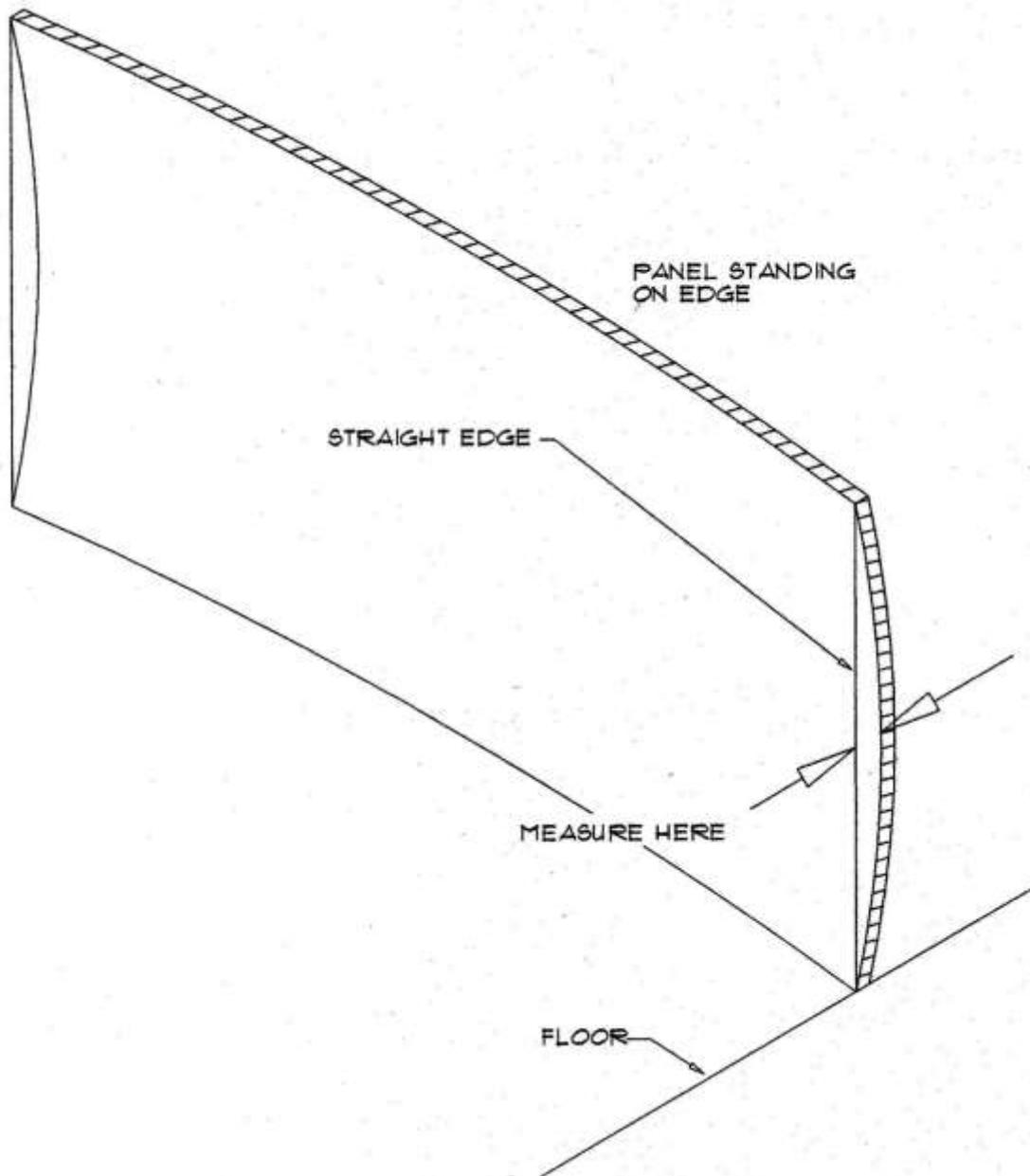
Figure 1. Example of cup measurement.
