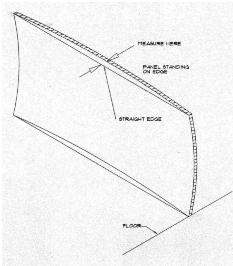
Figure 2. Example of bow measurement.
