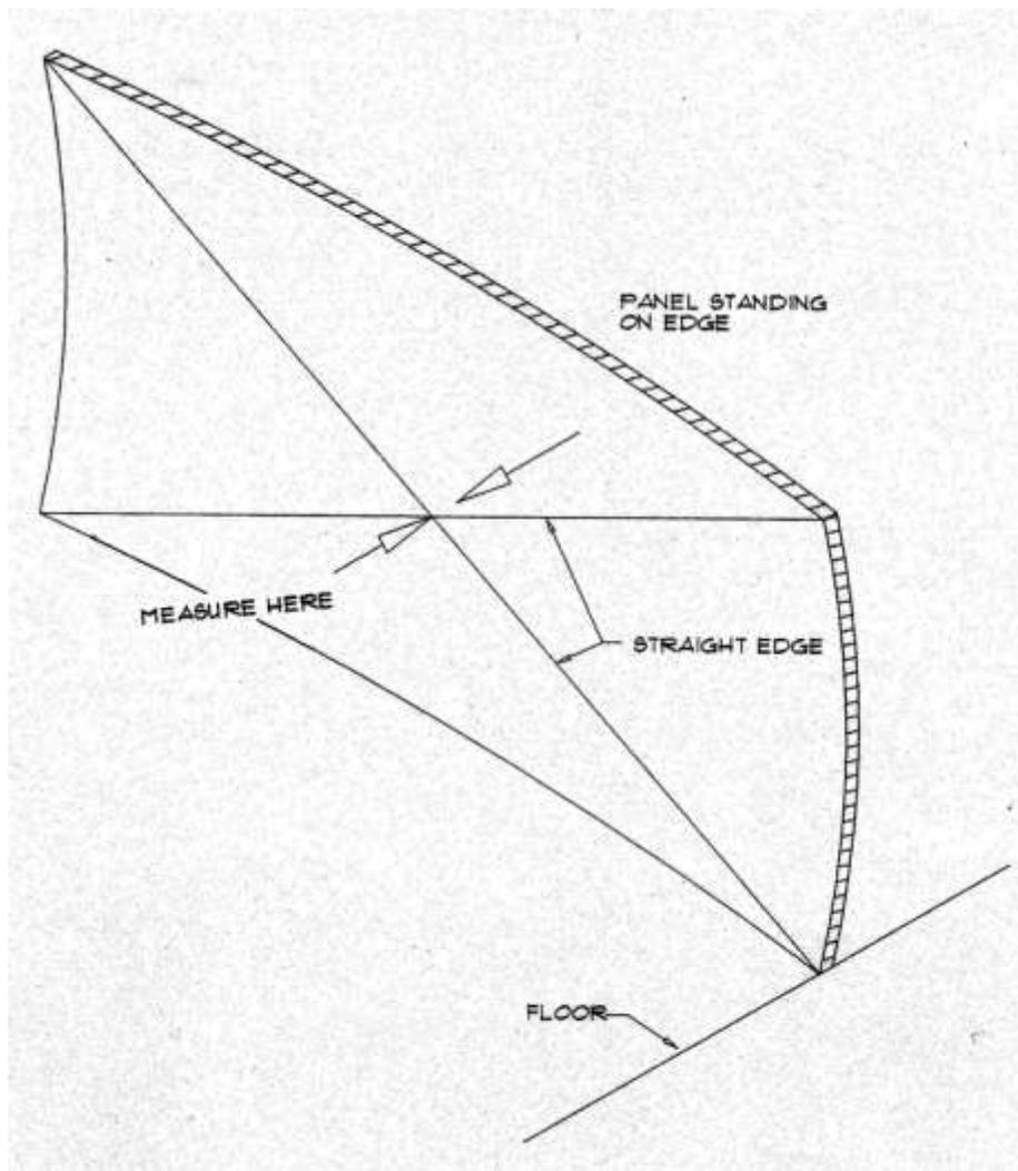
Figure 3. Example of twist measurement.
