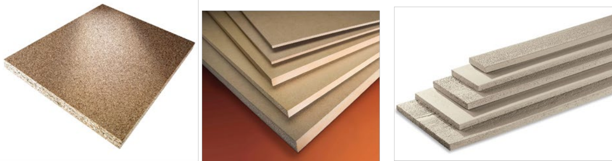
Figure 3. Particleboard, medium density, and hardboard/engineered wood siding and trim (EWST).
